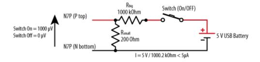
An alternative setup (that also avoids the polarity switch of the EEG channels that are referenced to the SRB2 pin) is below. Here it is harder to find out if a mastoid electrode (A1 or A2) was messed up or went bad:
