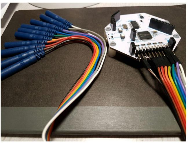
On the OpenBCI device, the Bottom pins are N pins, Top pins are P pins, so connect them in this way:
